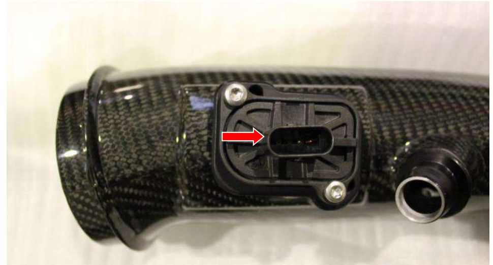
18. Insert MAF sensor into RHS tube – ensure that the sensor is oriented correctly . There is an arrow on the sensor indicating direction of airflow which is highlighted here in red. Secure both sensors with the supplied M4 torx screws.
