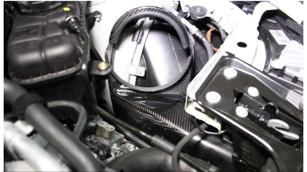
21. Take the right side duct (larger one) and locate the holes at the back over the holes shown previously on the stock duct opening. The new duct should go OVER the stock one.
