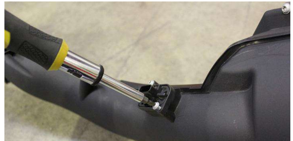
16. Using a Torx T20 – remove MAF sensors from both left and right side airboxes.
