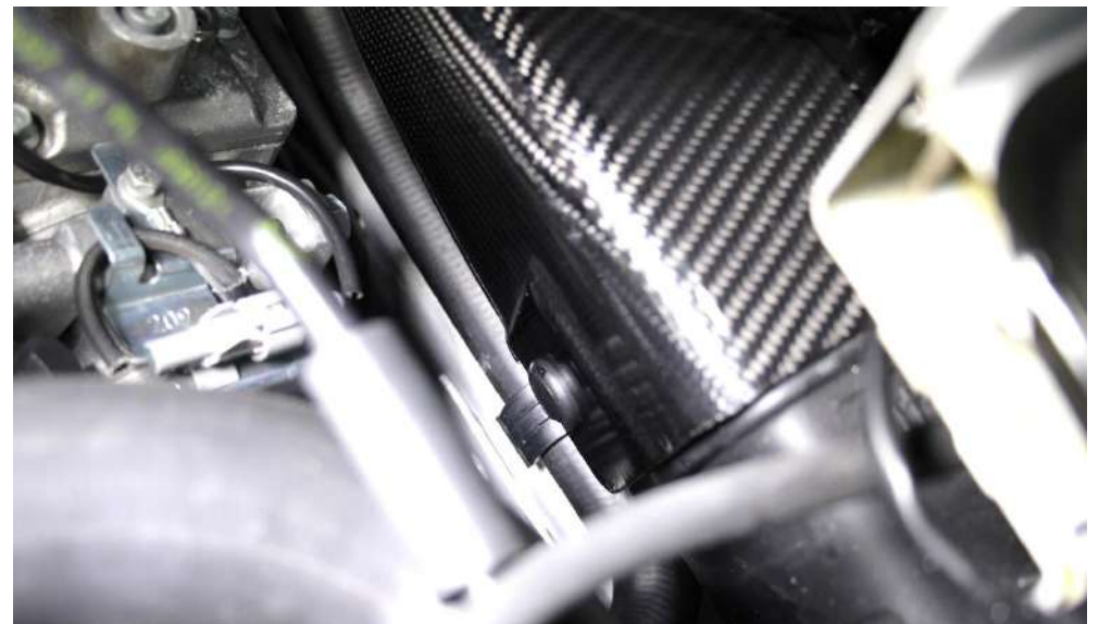
23. Starting on the side closes to the engine - align the hole on the new duct with the hole on the stock opening and push the rivet through. Secure by clicking the head in fully.
