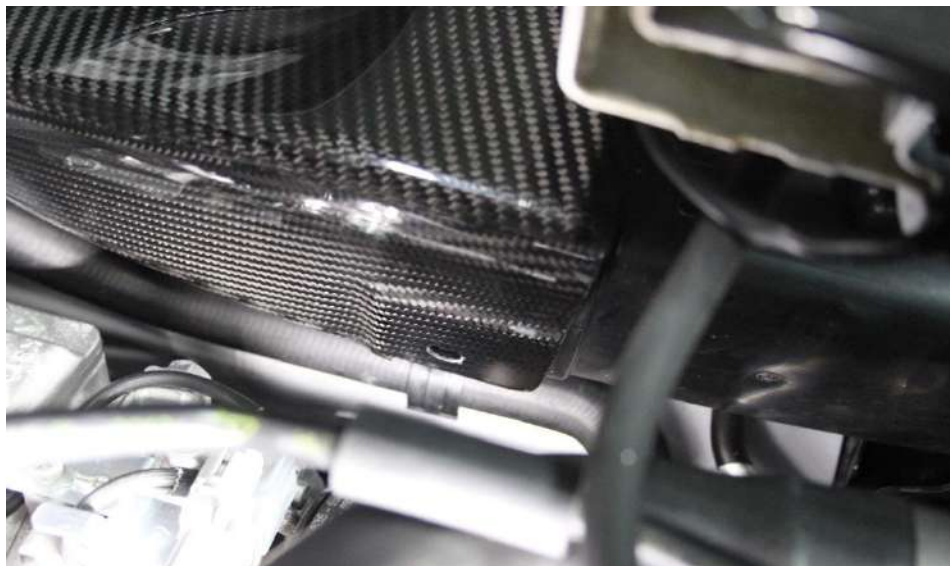
22. The right side duct should sit like this. Now secure it using 2 push rivets.....
